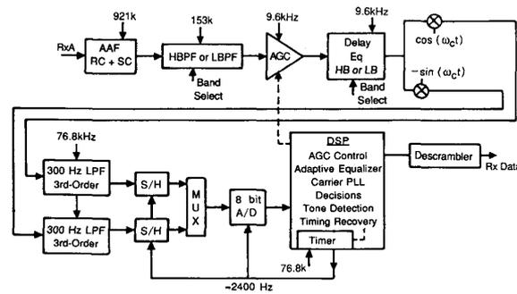
Fig. 5. Receive signal processing in the IC. SC clock frequencies are shown.
