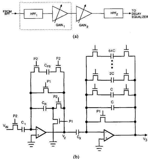
Fig. 8. (a) Programmable gain stage with HPF's. (b) Schematic of first half of programmable gain stage: input HPF and first gain amplifier.
