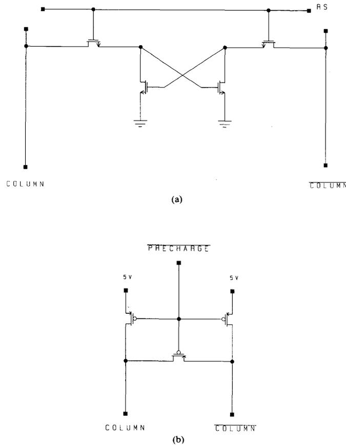
Fig. 10. Dynamic RAM: (a) four-transistor cell, and (b) column precharge. (Continued.)
