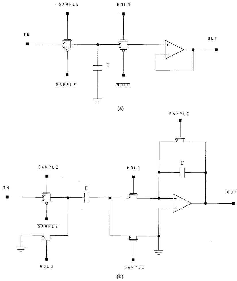
Fig. 7. (a) Conventional S/H requiring an op amp with large input common-mode range. (b) S/H with no input common-mode swing required of the op amp.
