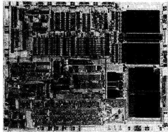
Fig. 13. Die photograph of the modem IC.
