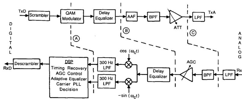
Fig. 2. Three different analog/digital partitionings.
