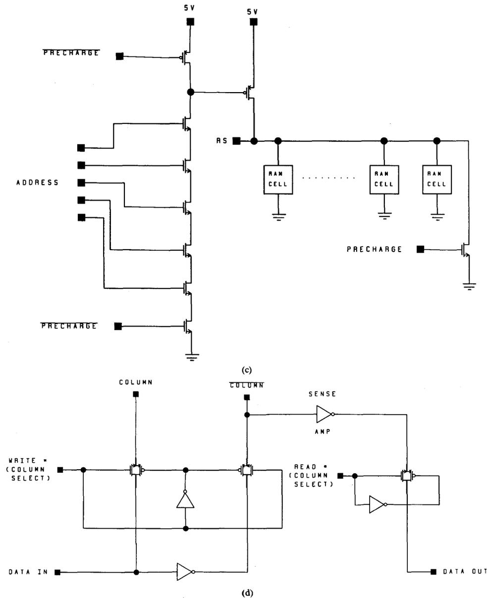
Fig. 10. (Continued.) Dynamic RAM: (c) address decoder with precharge, and (d) I/O circuitry.
