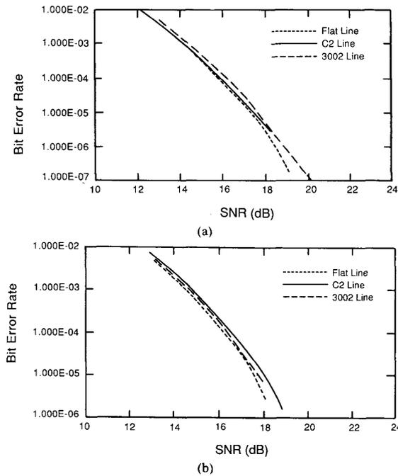
Fig. 12. 2400-b/s modem performance: bit-error rate versus input SNR. (a) Low band. (b) High band.
