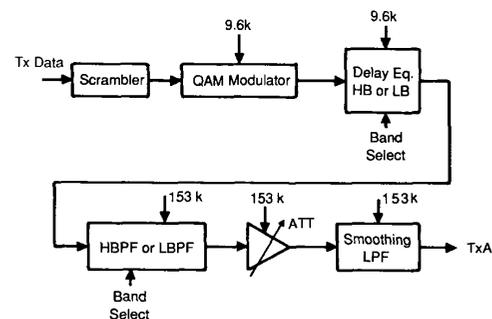
Fig. 3. Transmit signal processing. SC clock frequencies are shown.
