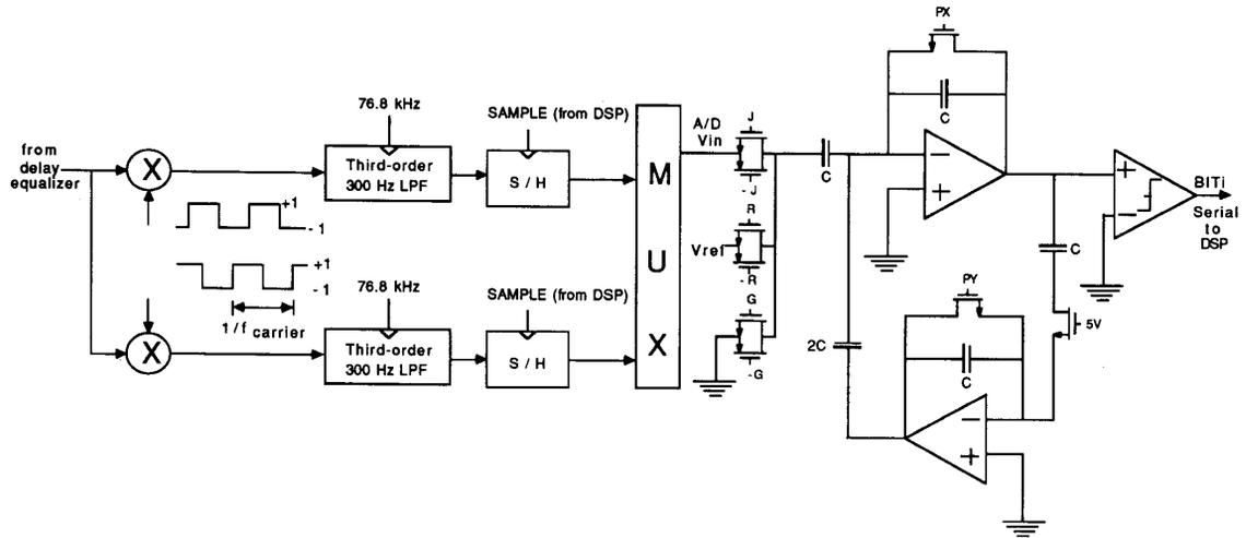
Fig. 6. Details of the fixed-frequency demodulator and 8-b ADC.
