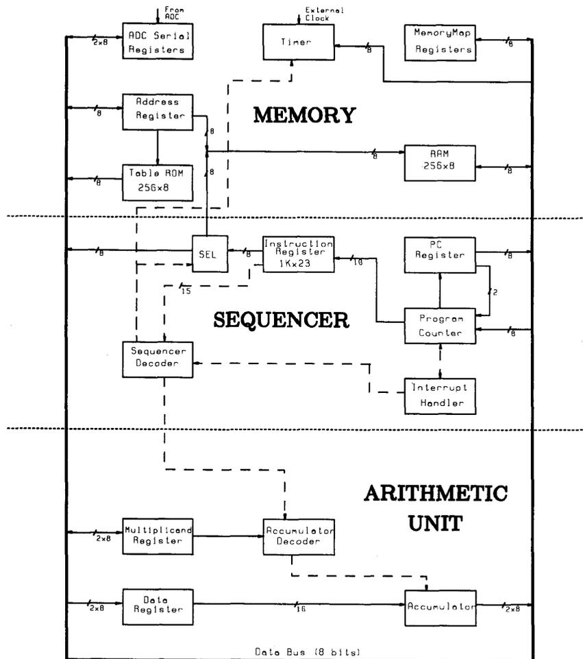
Fig. 9. DSP block diagram.
