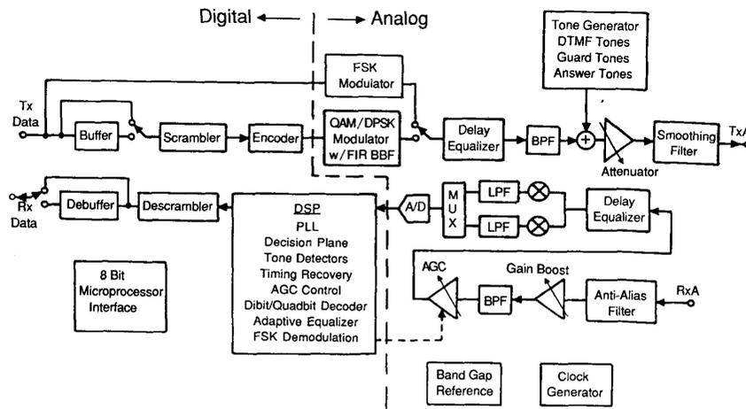
Fig. 1. V.22bis modem IC block diagram, showing the analog/digital partitioning.
